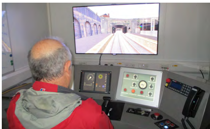
Facilities in the system integration lab have allowed extensive pre-installation testing. Top, a driver's eye view of Farringdon station created by the simulator. Above left, Rod Muttram takes the controls of the simulated train. Above right, a balise reader (inverted) in its test rig.
