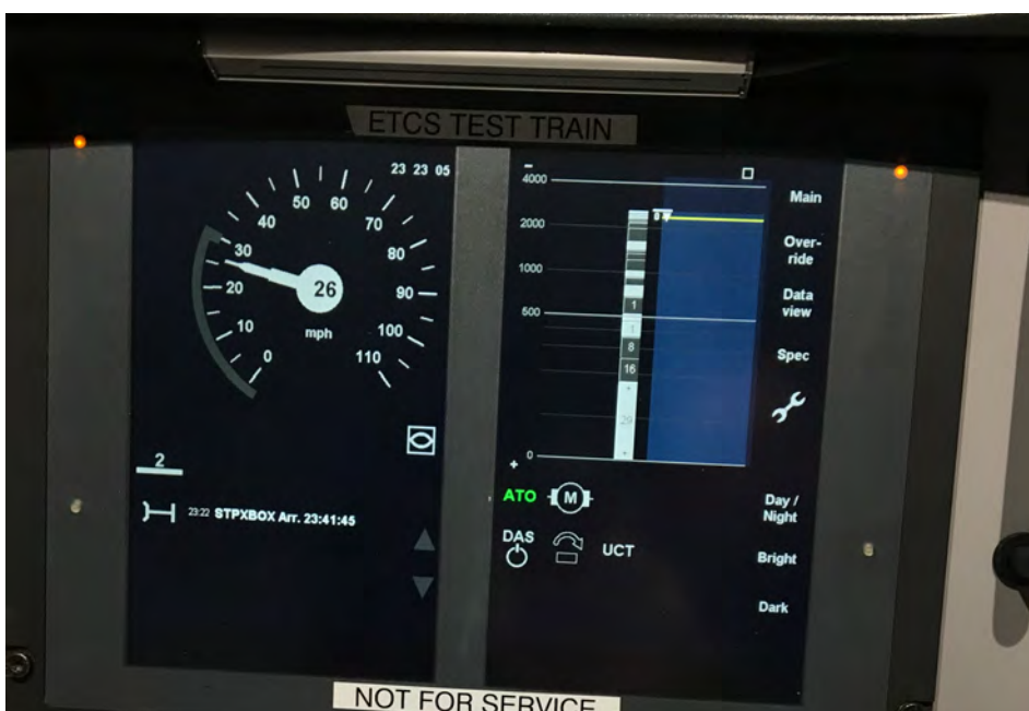
Figure 3 – Thameslink Class 700 – the DMI display operating in ATO.
