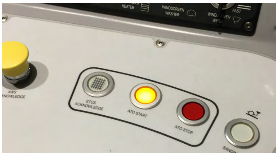
Figure 4 – Thameslink Class 700 ETCS and ATO Controls in the cab.
