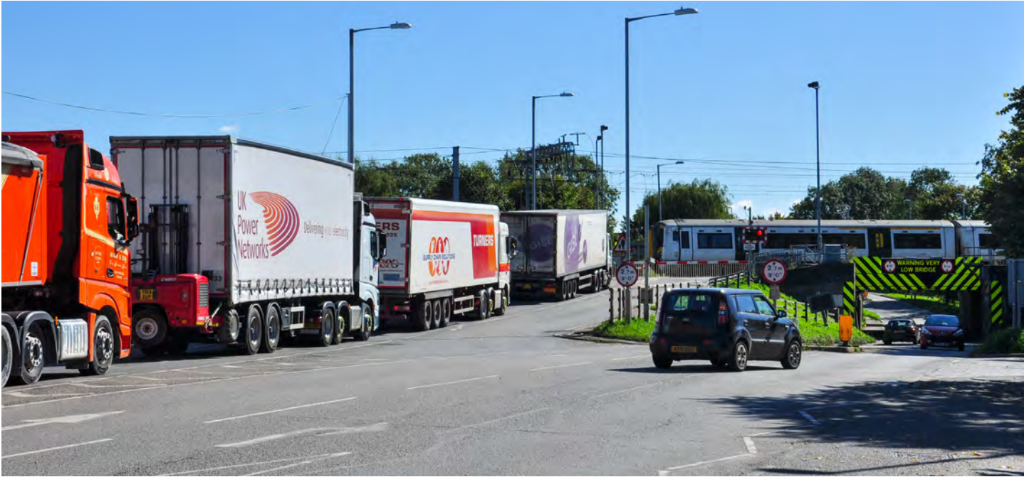
Figure 2 – More use of a level crossing by heavy road vehicles is an example of how a residual risk could be increasing even when there are no changes to the railway.
