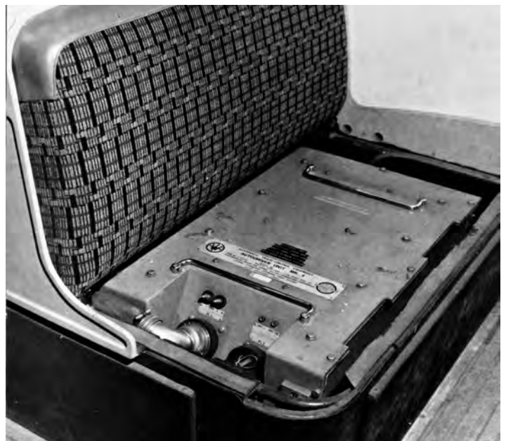
The original Victoria Line Autodriver (above) sat under a passenger seat in the saloon, and was a masterpiece of 1960s electronics as seen in the detail shot of the unit in the museum (top left). Later versions of the autodriver are shown in the photo on the left. Original 1968 photo Westinghouse archive.
