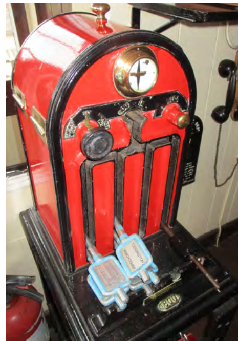
The Toddington to Winchcombe token machine at Toddington. Photo Clive Kessell.
