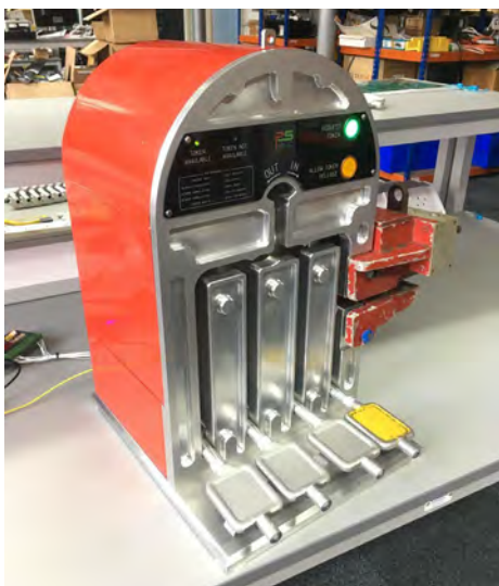
DiBLoC, a modern replacement for the Tyer’s token instrument.
