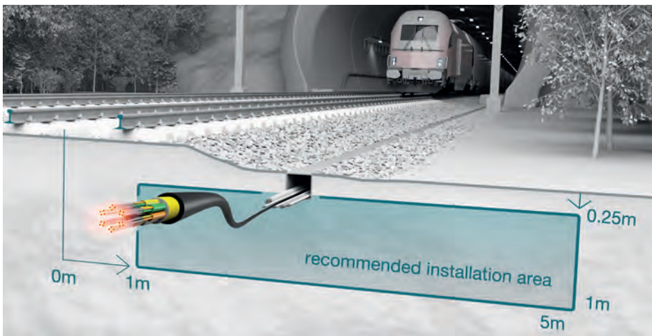
Figure 4 – Fibre optic cables are often already in place along a track and can be used to install FTS.
