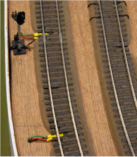
Figure 2 – Hall effect sensors are placed at braking distance before each signal.
