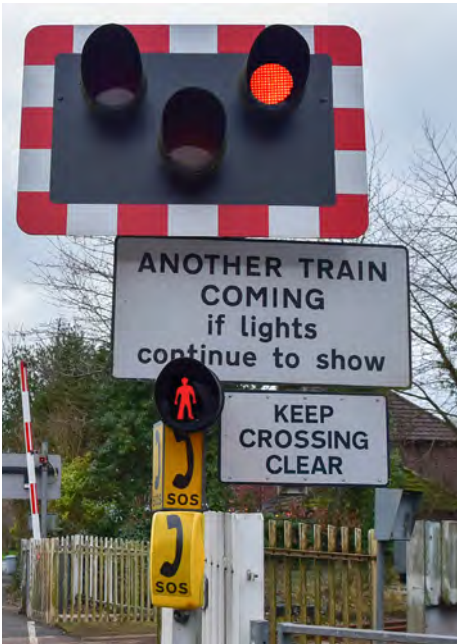
Figure 2 – 'standing red person' signal (centre) supplementing road lights.
