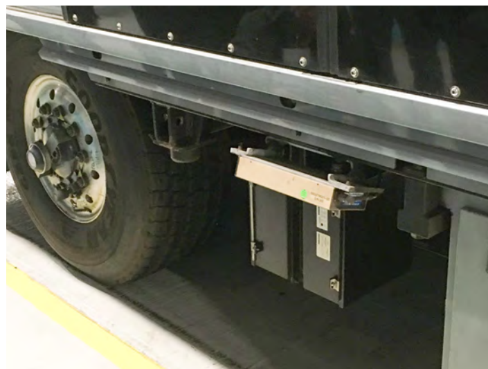
Innovia 200 wheel and tyre and the CBTC Radiax antenna mounted on the solebar
