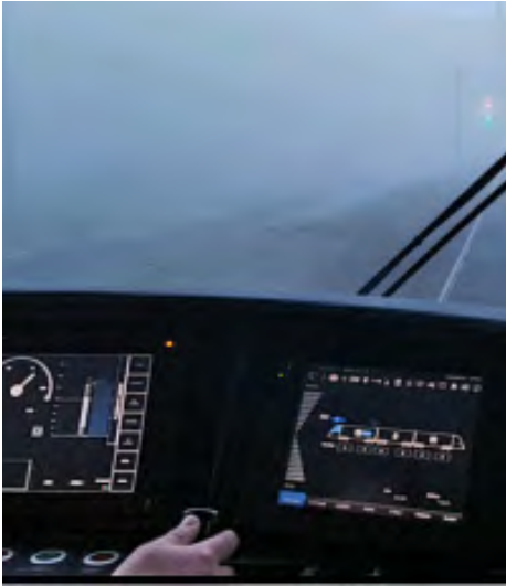
Figure 4 – Accelerating into the fog. The driver is about to pass a signal for which there will be less than 5 seconds sighting at full line speed. Can you see it?
