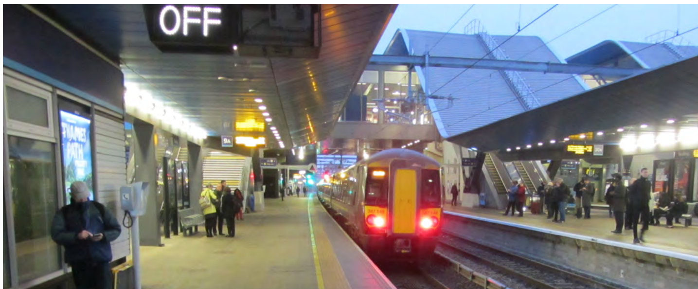
Reading Down Main platform is almost straight, with the green LED signal beyond the platform ramp readable by drivers at 95mph (155km/h), yet it has three Off indicators.
