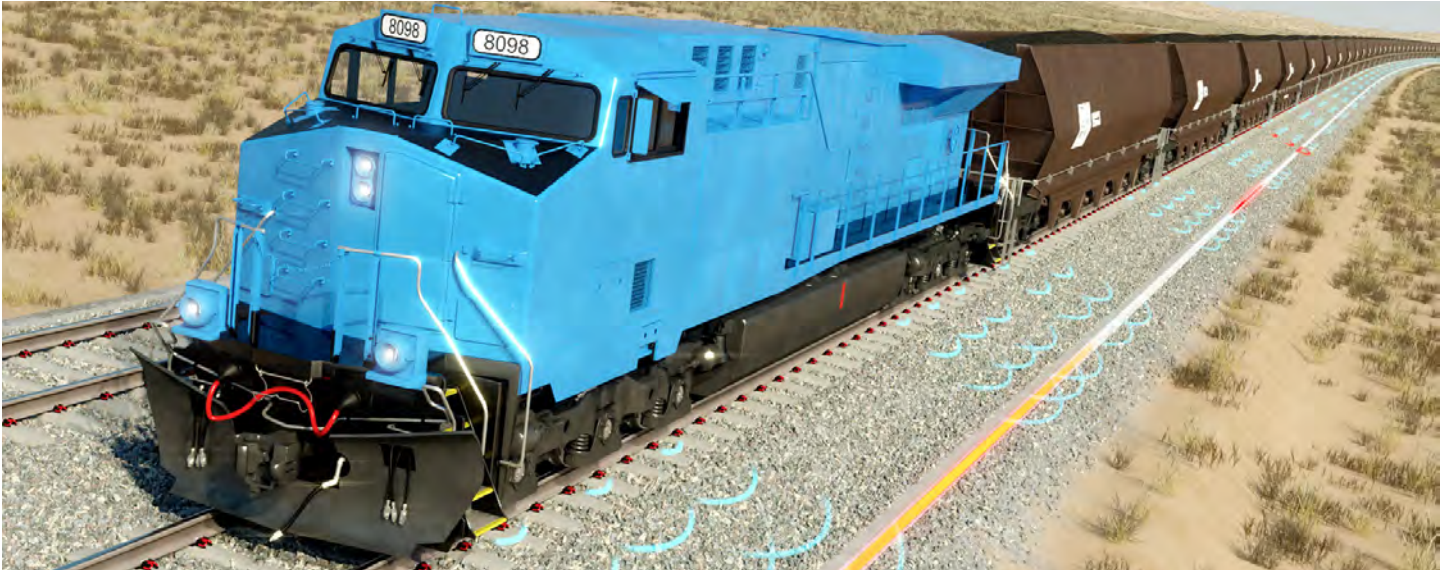
Figure 3 – Trains can be detected by DAS within a maximum radius of 50 metres.
