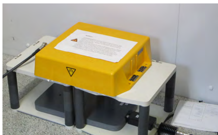
Facilities in the system integration lab have allowed extensive pre-installation testing. Top, a driver's eye view of Farringdon station created by the simulator. Above left, Rod Muttram takes the controls of the simulated train. Above right, a balise reader (inverted) in its test rig.
