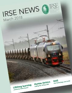
Our cover photo shows a freight train operated by mining company LKAB over the route from Kiruna, Sweden to the Baltic at Luleå and Atlantic Coast at Narvik, Norway. Trains are controlled with the assistance of Driver Advisory Systems (DAS). Each 750 m train consists of 68 ore cars, carrying up to 6,800 tonnes of iron ore.
