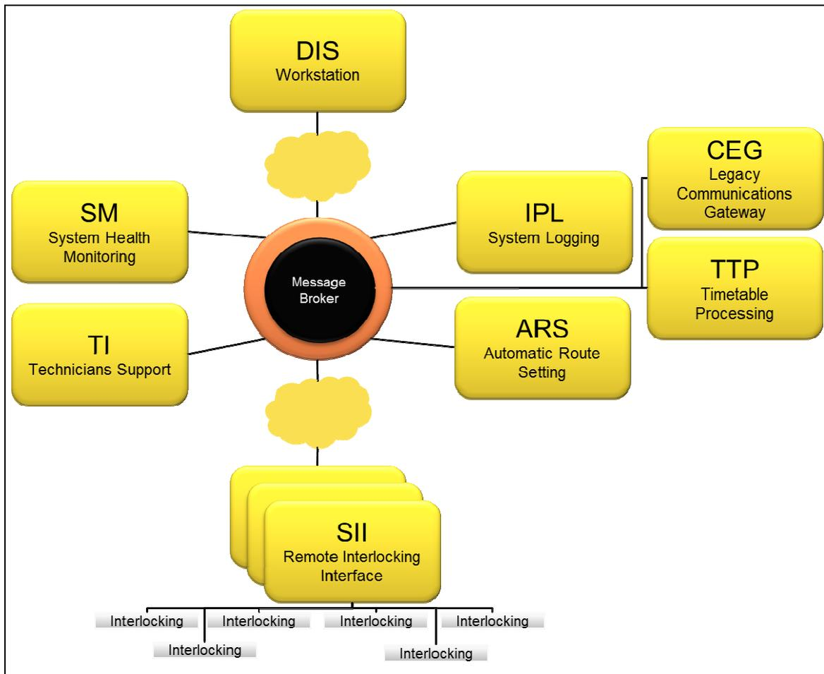
Figure 1 An Overview of the IECC Scalable Architecture
